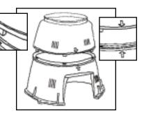
Step 3 – Check the outside and inside with your hand to ensure the 6 tabs line up with the 6 slots.
